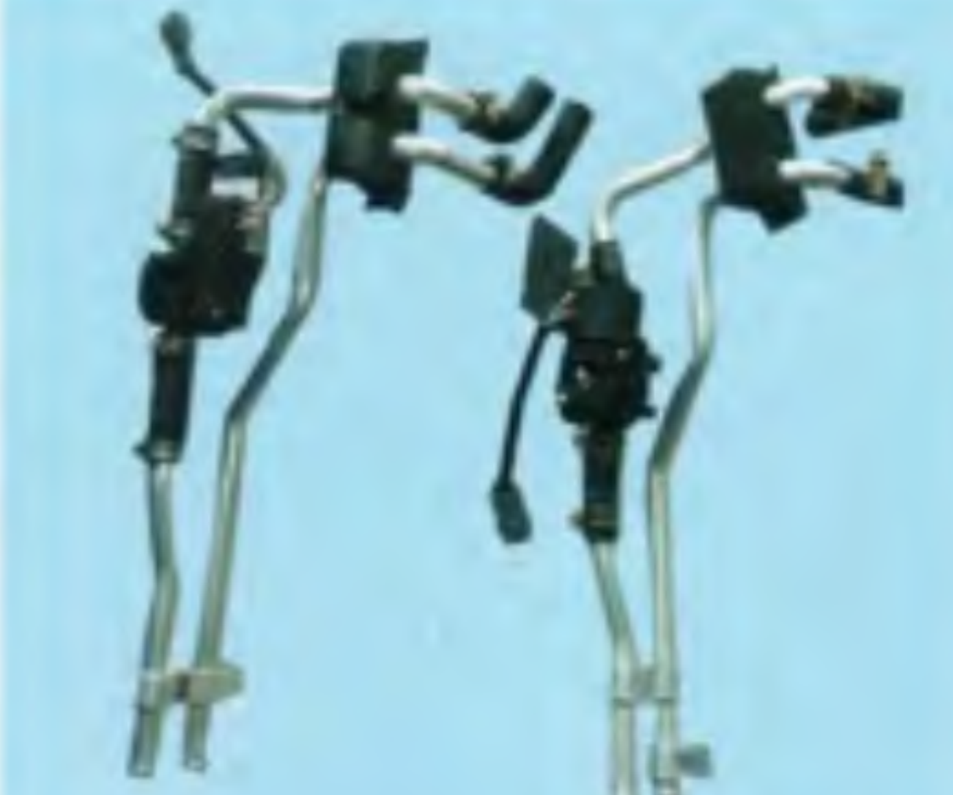
Warm-Water Pipe Assemble
